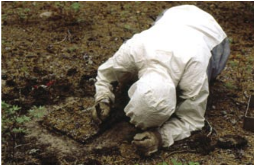
Figure 9. The fire-fuel properties of the forest floor layer in the International Crown Fire Modelling Experiment study area were determined from 30 x 30 cm samples taken down to the mineral soil.
