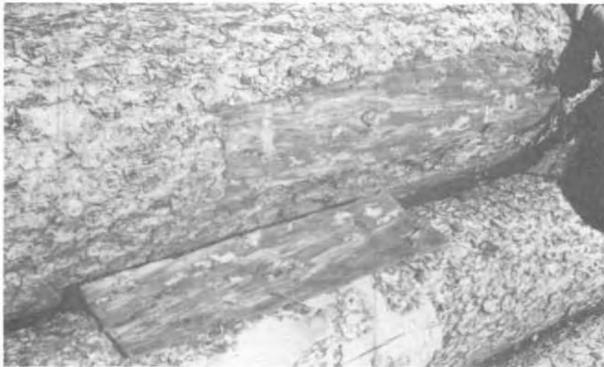
Figure 2. One square foot bark sample removed from white spruce log, exposing Tetrodium attack.
