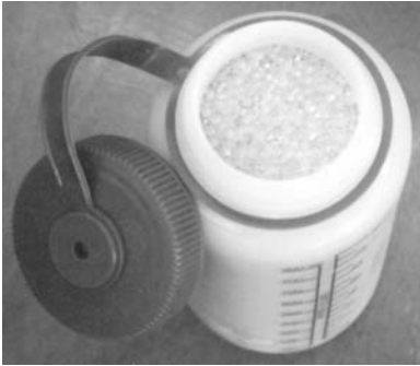
Photo 3 3-mm glass beads used in the field for volume measurement of excavated soil samples.
