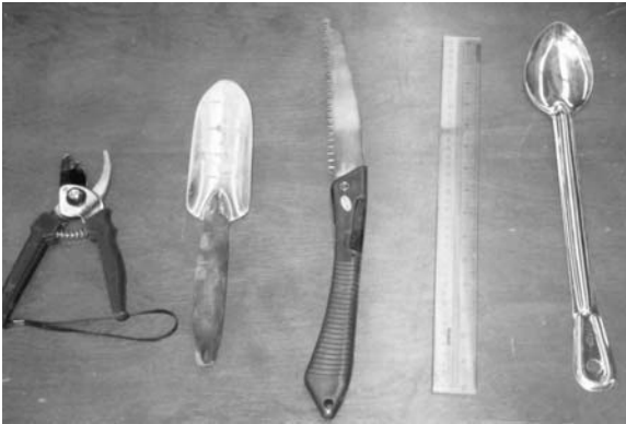
Photo 1 From left to right: hand clippers (for clipping fine roots and shrubs, herbs and grasses at the microplot); hand trowel; folding aluminum hand saw (for cutting forest floor organic sample); ruler and long-handled, stainless steel soup spoon (for scooping finely textured soil at successive depths).
