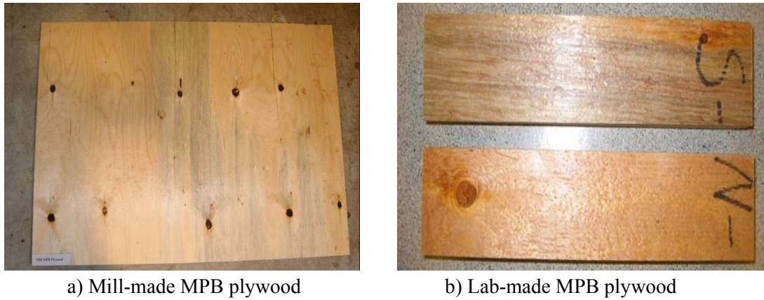
Figure 15. The appearance of mill and laboratory made MPB plywood.
