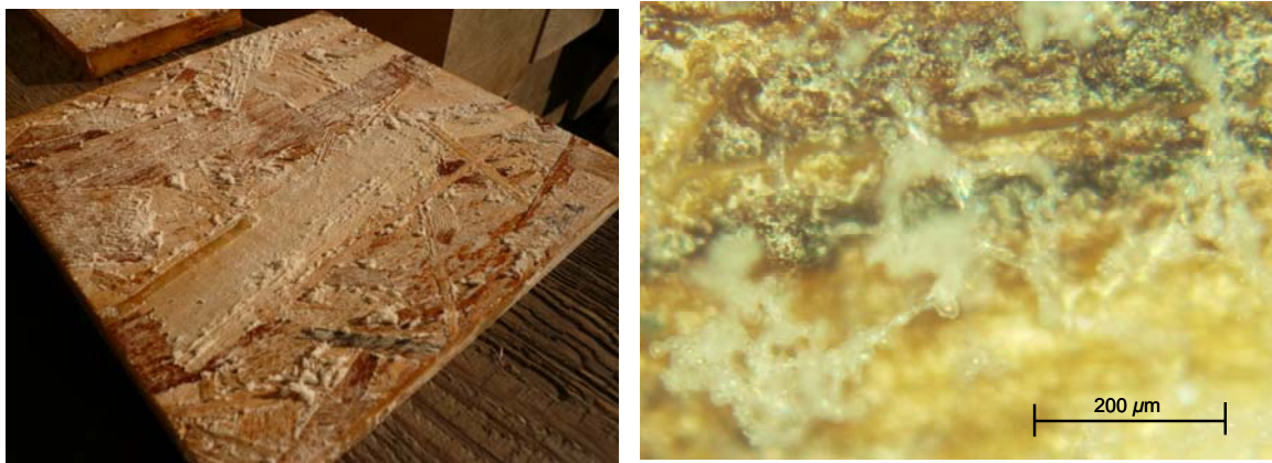
Figure 26. (a) Expanded microspheres (20 \mu\text{m} unexpanded) on a treated and dried OSB surface, and (b) magnified 20X.
