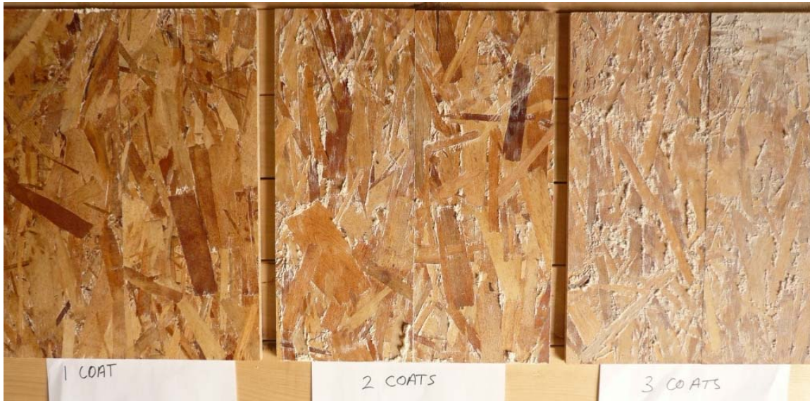
Figure 37. The outcome of roller coating boards with one pass, two passes, and three passes with a mixture of expanding microspheres and PF resin at 20% solids content.
