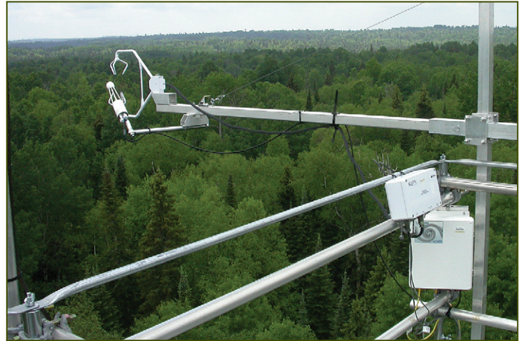
Image 3. Gas analyzer and sonic anemometer on McKeown Lake tower, above mature boreal mixedwood forest.
