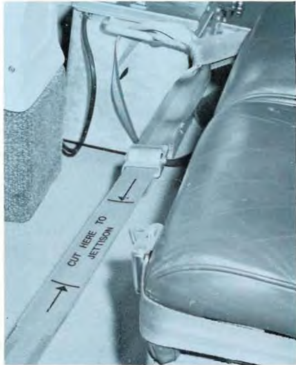
Figure 7. Inboard end of tie-down strap showing jettison label and forward restraint.
