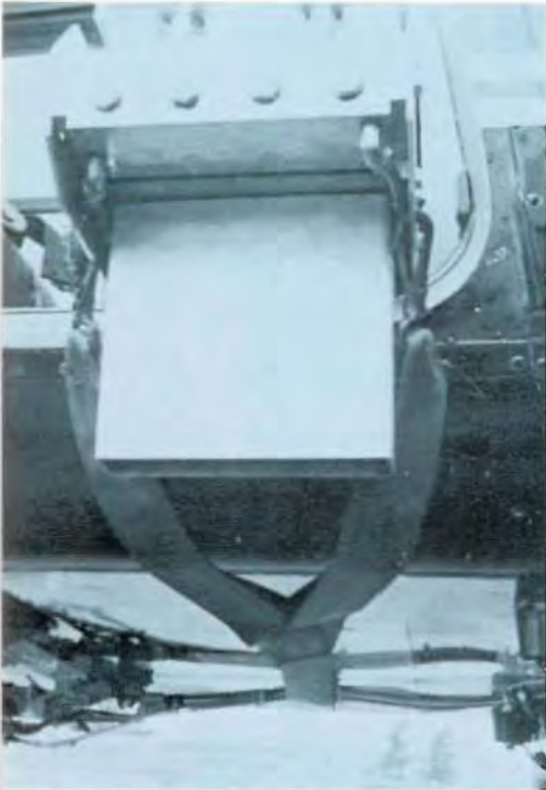
Figure 6. Outboard end of tie-down strap under aircraft cabin.
