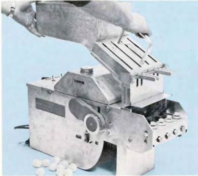
Figure 8. Removal of hopper and feed chute assembly.
