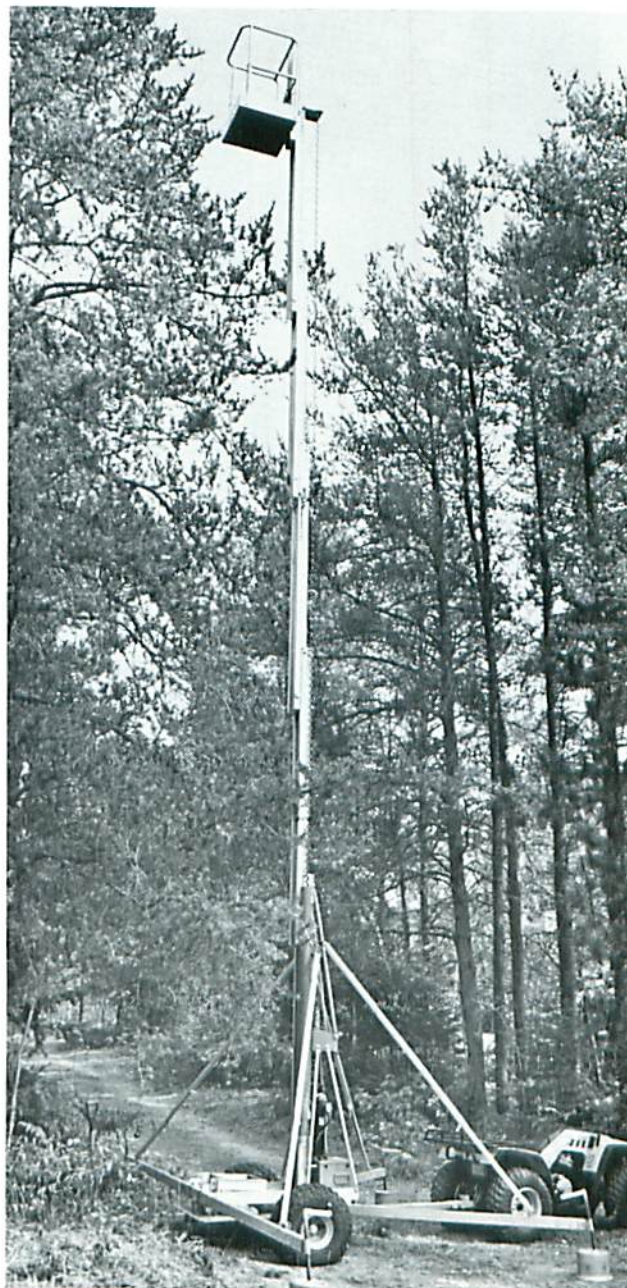
Figure 1. Portable personnel lift system used to assess the upper crown levels of trees.
