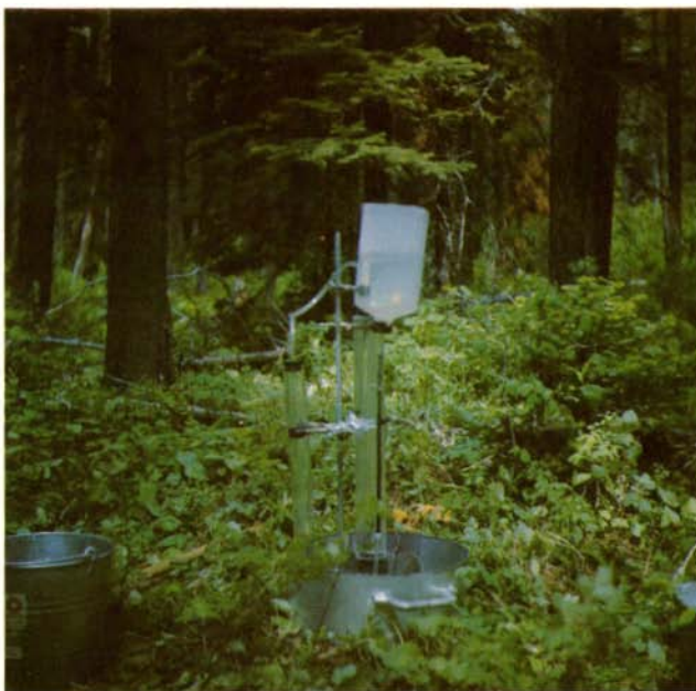
Figure 29. Field testing of water infiltration rates.
