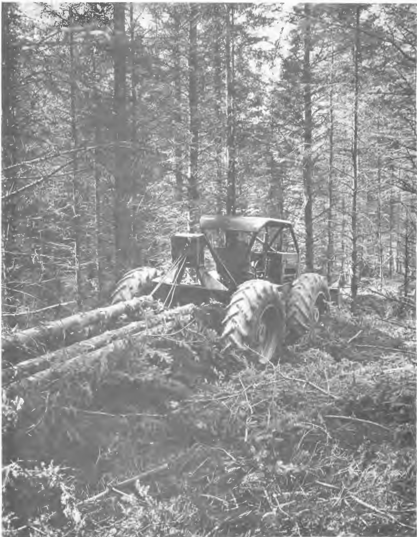
Skidding tree-lengths in white spruce plantation row-thinning. Petawawa Forest Experiment Station. Canadian Forestry Service photo.
