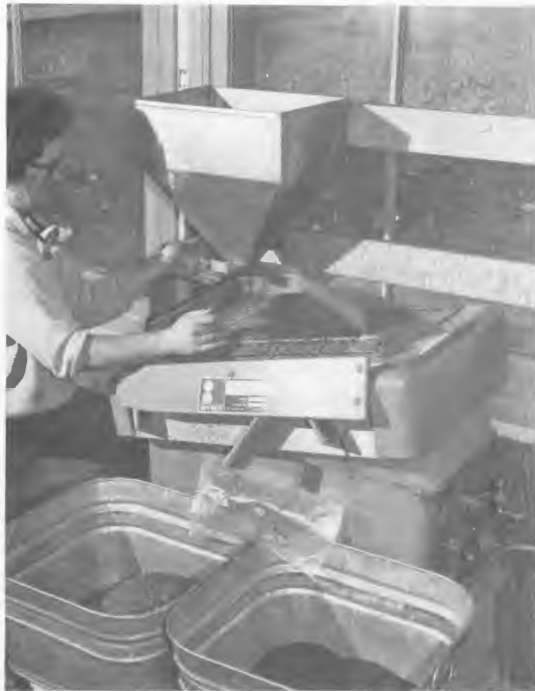
Specific gravity table for final seed cleaning. Duncan, B.C. B.C. Forest Service photo.
