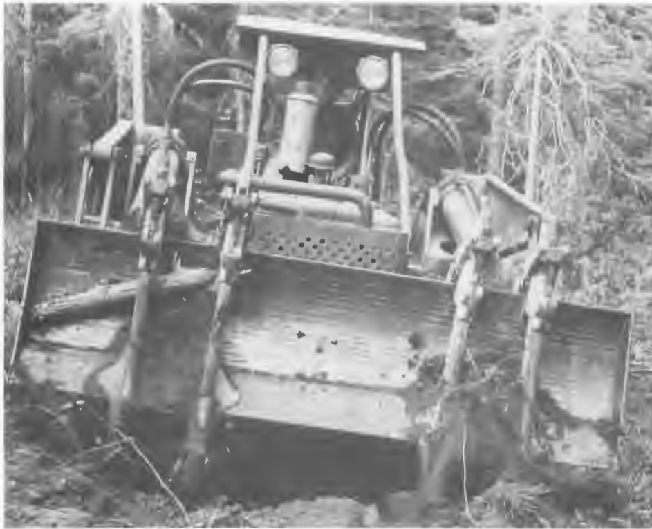
Scarifying clearcut strip with blade and ripper teeth. Aleza Lake, B.C. B.C. Forest Service photo.
