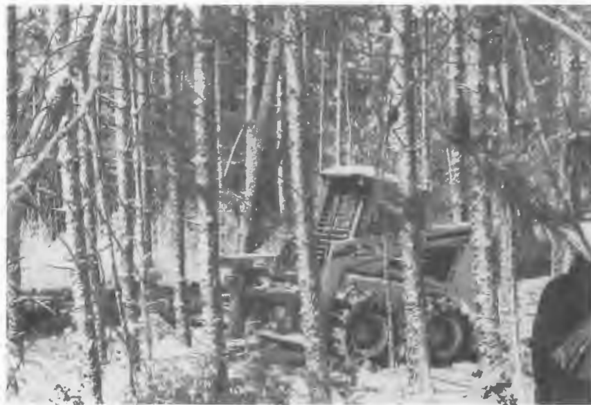
Melrose Bobcat feller buncher, with Morbark shear, row-thinning red pine plantation. Petawawa Forest Experiment Station. Canadian Forestry Service photo.
