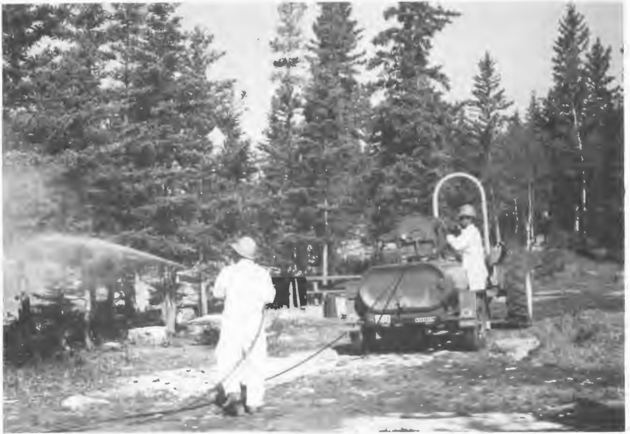
Spruce budworm control with trailer-mounted hydraulic sprayer. Rocky Lake, Man. Canadian Forestry Service photo.
