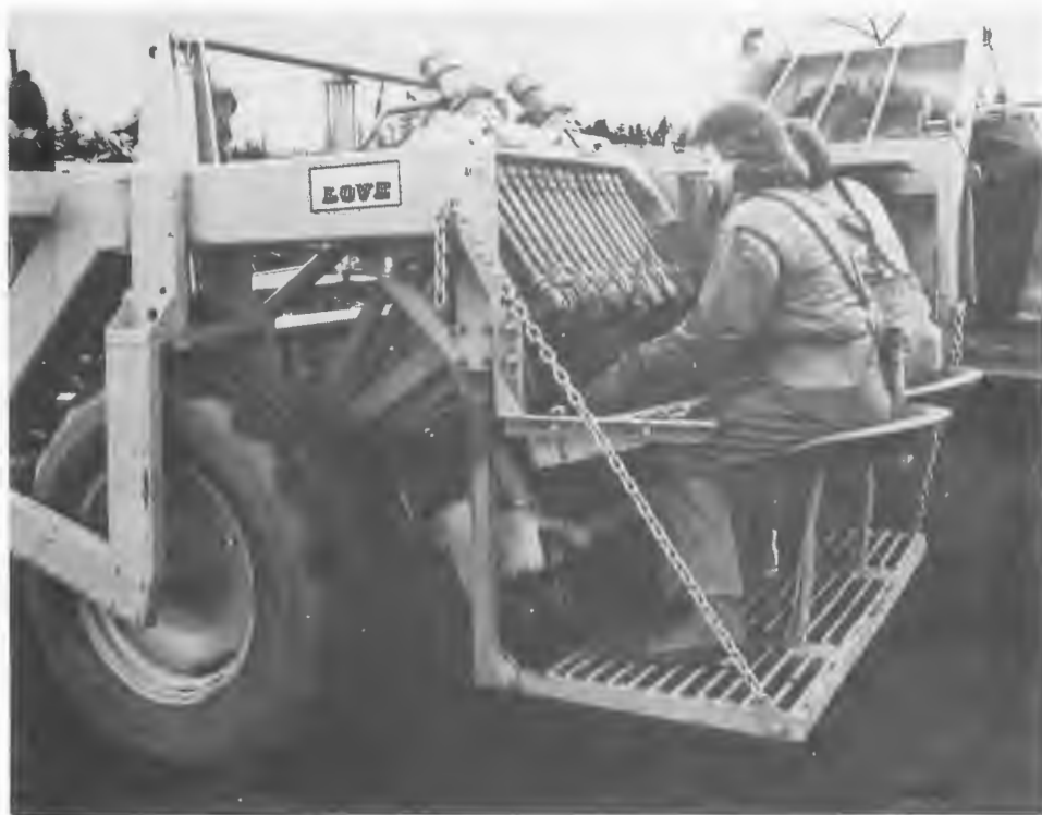
Love machine for lifting seedlings. Surrey Nursery, B.C. B.C. Forest Service photo.
