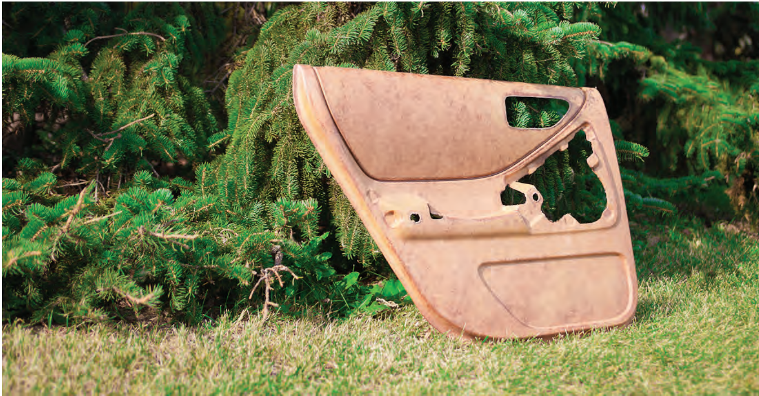
An engineered wood fibre mat could replace fibreglass components in cars.
