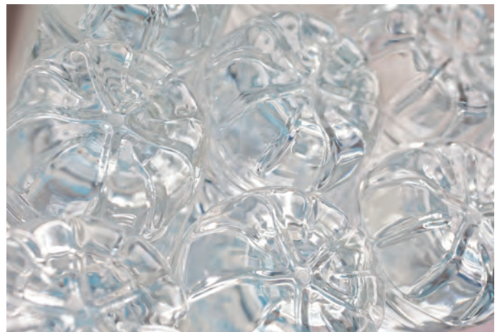
Biomaterials such as cardboard and sawdust can be used to create bio-polyethylene terephthalate (bio-PET), a component in traditional plastic soda bottles.
