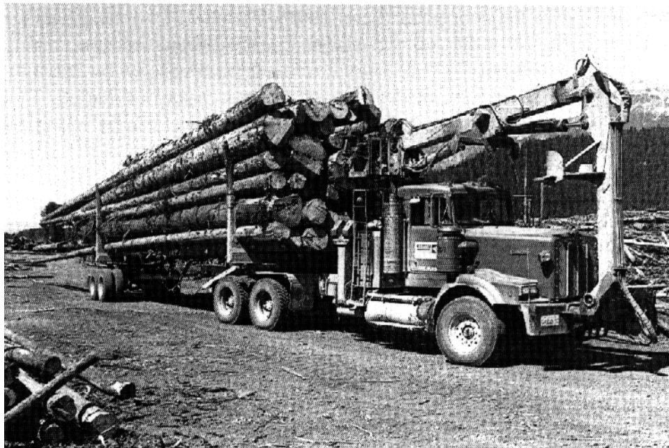
Figure 1. Barko 145A log loader mounted on a Kenworth C5000 log-hauling truck.
