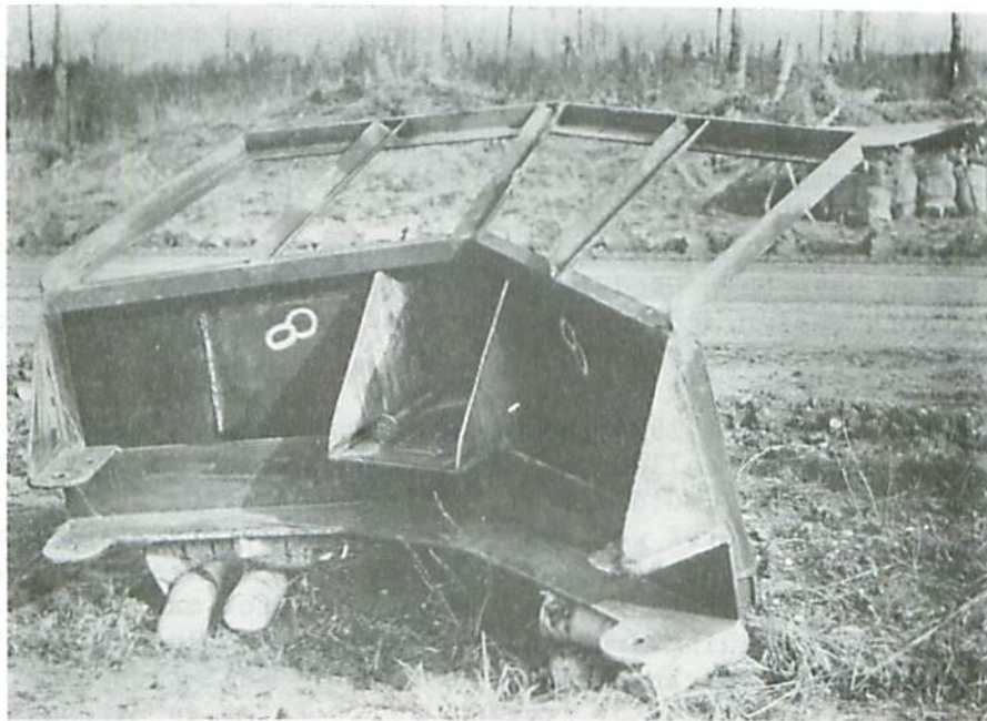
Fig. 3. V blade showing "butt plate and lips" method of attachment to tractor C frame.
