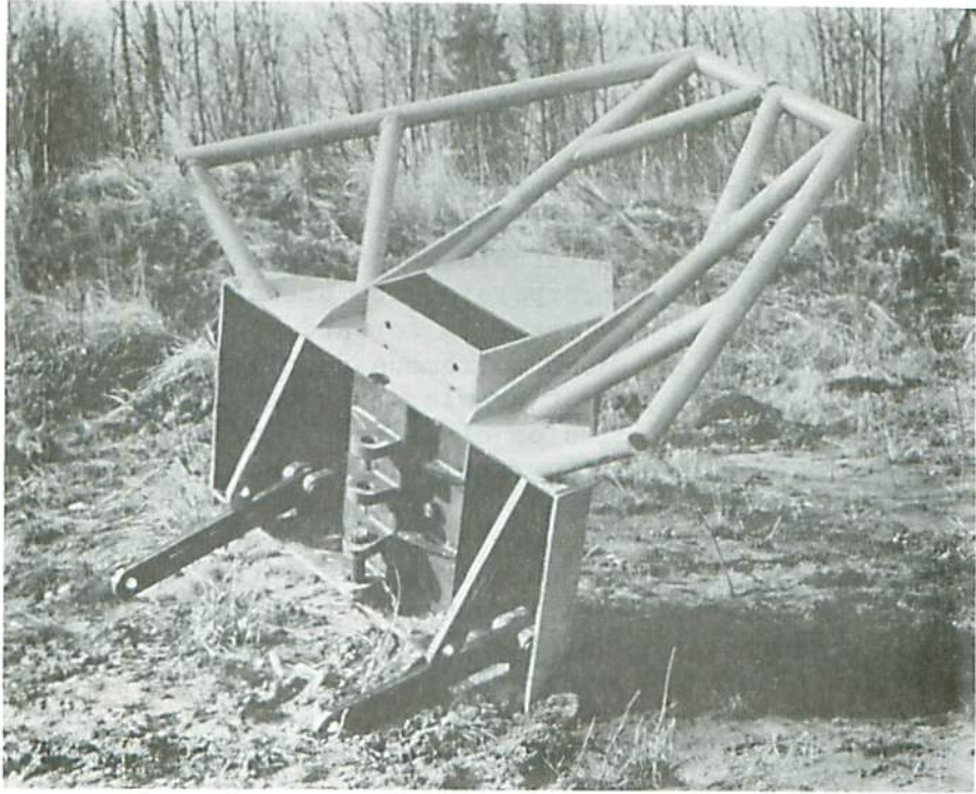
Fig. 4. CFS V blade showing method of attachment.
