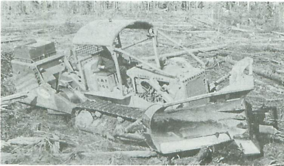
Fig. 7. Taylor Drum planter mounted on Cat D6B bulldozer. Note debris passing under wings of V blade while scalping foot clears necessary path.
