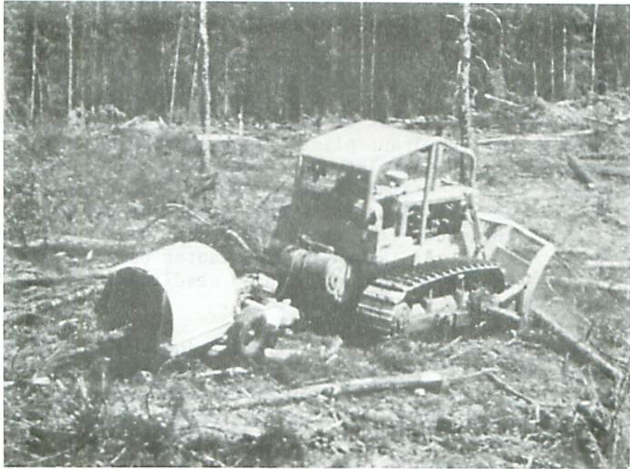
Fig. 2. Crank Axle planter drawn by Cat D6C bulldozer. Note trunnion arms on curved face of V blade.
